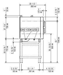
Cold Water inlet 1 (cleaning) CWII Cold Water Inlet 2 (steam CWI2 generator)
